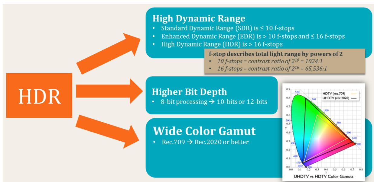
Figure 2: Components of HDR technology
