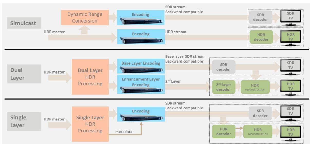
Figure 5: Backward Compatibility implementations in HDR delivery chain
