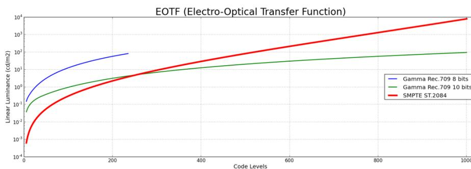
Figure 3 : EOTF examples - SMPTE ST.2084 vs. Gamma
