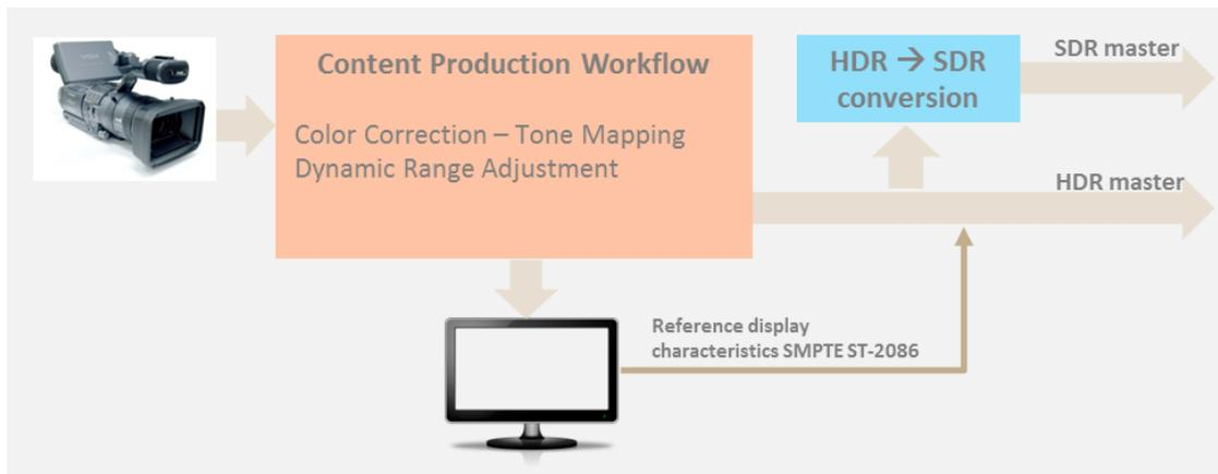
Figure 4: Content Production Workflow
